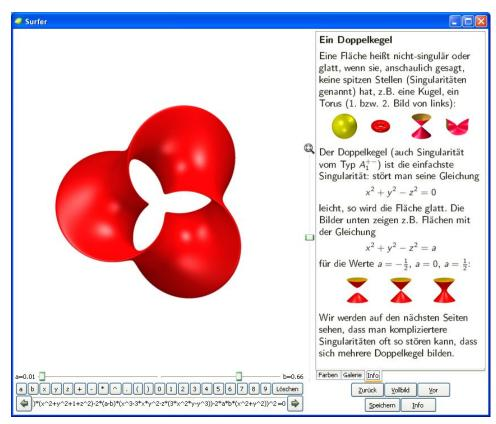
In our case, the formulas contain the two variables a, b which control the axes of the rotating ellipse. The scroll bar allows the fixing of values from 0 to 1. The parameter values a = 0 or b = 0 produce singular results and lead to visualisation errors with the SURFER. Therefore it makes sense to add a small offset to the parameter a, e.g. replace a by 0.01 + a. If one is interested in self-intersections, one can also use larger parameters by 2a.
